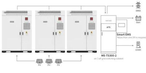
Application scenarios of energy storage battery products
