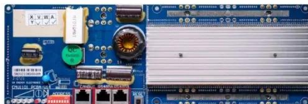
BS485 Communication between battery and inverter Band rate: 9600bps BS485 Interface Communication between parallel packs of BMS and PC Band rate: 9600bps
